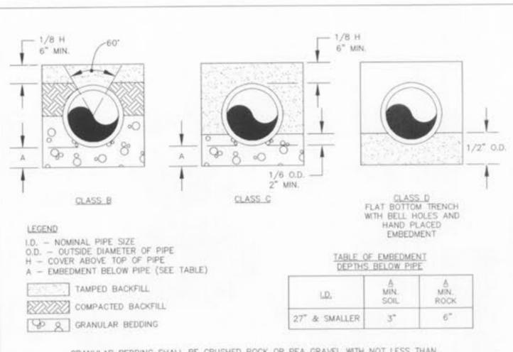
GRANULAR BEDDING SHALL BE CRUSHED ROCK OR PEA GRAVEL WITH NOT LESS THAN 95% PASSING 1/2" (95% PASSING 3/4" FOR 30" AND LARGER PIPE) AND NOT LESS THAN 95% RETAINED ON A #4: TO BE PLACED IN NOT MORE THAN 6" LAYERS AND COMPACTED BY SLICING WITH A SHOVEL OR VIBRATING.
