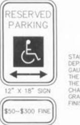
STANDARD SIGN FACE, STANDARD HIGHWAY DEPARTMENT, OR CITY STREET DEPARTMENT GAUGE, LETTERS AND BORDERS ARE GREEN, THE HANDICAP LOGO SQUARE IS BLUE AND THE BACKGROUND IS WHITE, GALVANIZED U CHANNEL POST 8'-0" LONG, SET 3'-0" INTO GRADE, SET BOTTOM OF SIGN 5'-0" ABOVE FINISHED GRADE.
