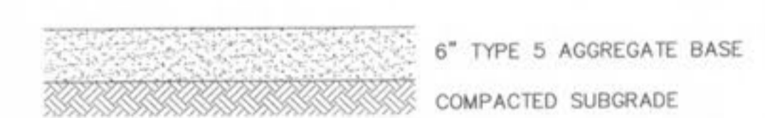
GRAVEL SECTION — DRIVEWAY NOT TO SCALE
