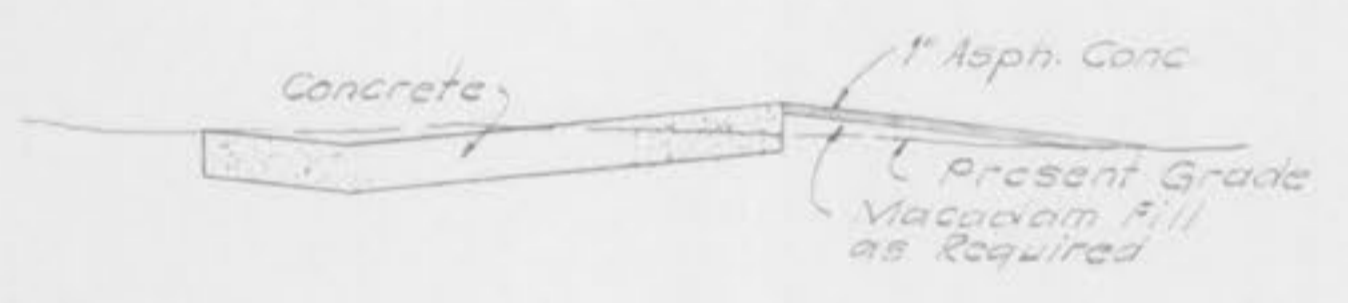
SECTION 2 (DRIVEWAYS IN CUT SECTION) Scale: 3/8" = 1'-0"
