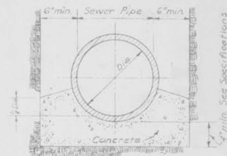
CONCRETE SEWER CRADLE
