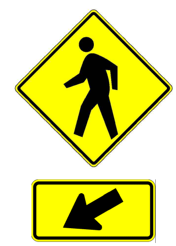
W11-2 "PEDESTRIAN CROSSING" SIGN OVER W16-7PL "DIAGONAL ARROW" SIGN NOT TO SCALE
