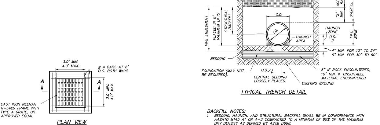
BEDDING, HAUNCH, AND STRUCTURAL BACKFILL SHALL BE IN CONFORMANCE WITH AASHTO M145 A1 OR A-3 COMPACTED TO A MINIMUM OF 95% OF THE MAXIMUM DRY DENSITY AS DEFINED BY ASTM D698.
