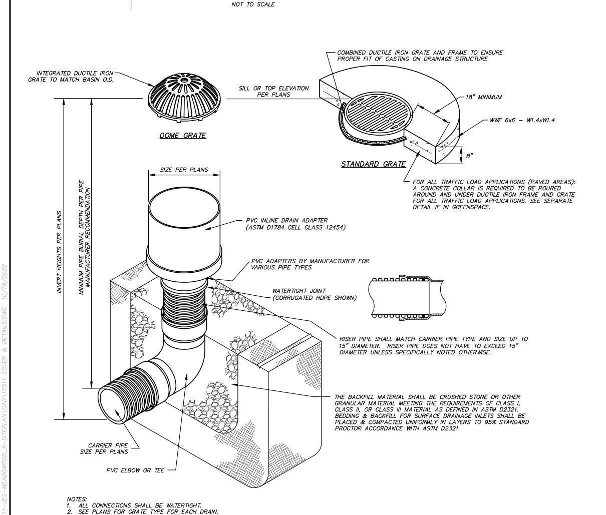
5. DRAIN ADAPTER SHALL BE CUSTOM MANUFACTURED AS A SINGLE UNIT ACCORDING TO PLAN DIMENSIONS. RISERS SHALL NOT BE ALLOWED WITHOUT PRIOR
