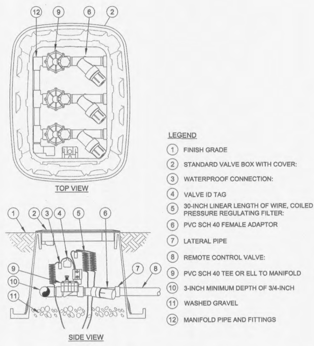
B DRIP ZONE KIT IN SQUARE VALVE BOX SCALE: N.T.S.
