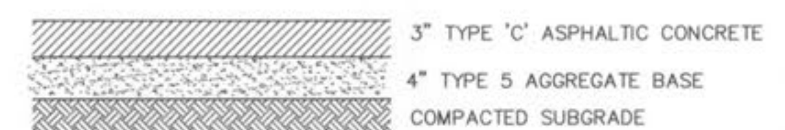
SIDEWALK SECTION NOT TO SCALE
