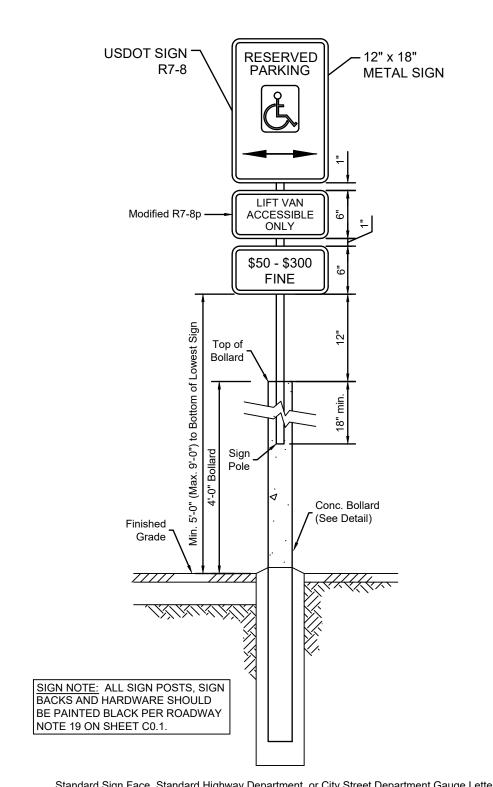
Standard Sign Face, Standard Highway Department, or City Street Department Gauge, Letters and Borders. The Galvanized U Channel Post, Set 18" into Bollard. Set the Bottom of the lowest Sign to a minimum of 5'-0" Above Finished Grade. Use "Lift Van Accessible Only" Sign Only when Applicable. Sign Should be Centered within 8' wide Parking Space.
