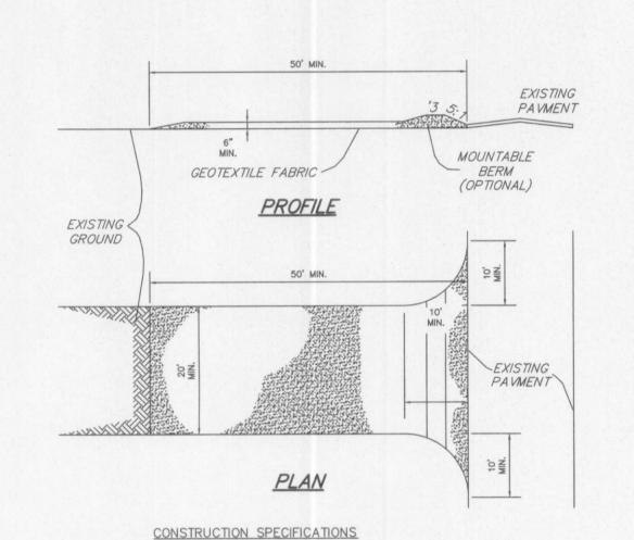
1. Stone Size — Use 2" stone, or reclaimed or recycled concrete equivalent.
