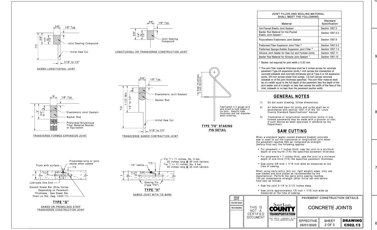
JOINT FILLER SHOWN ON DETAILS SHALL BE: SELF LEVELING CAULKING (SIKAFLEX - 2C - SL) OR APPROVED EQUAL
