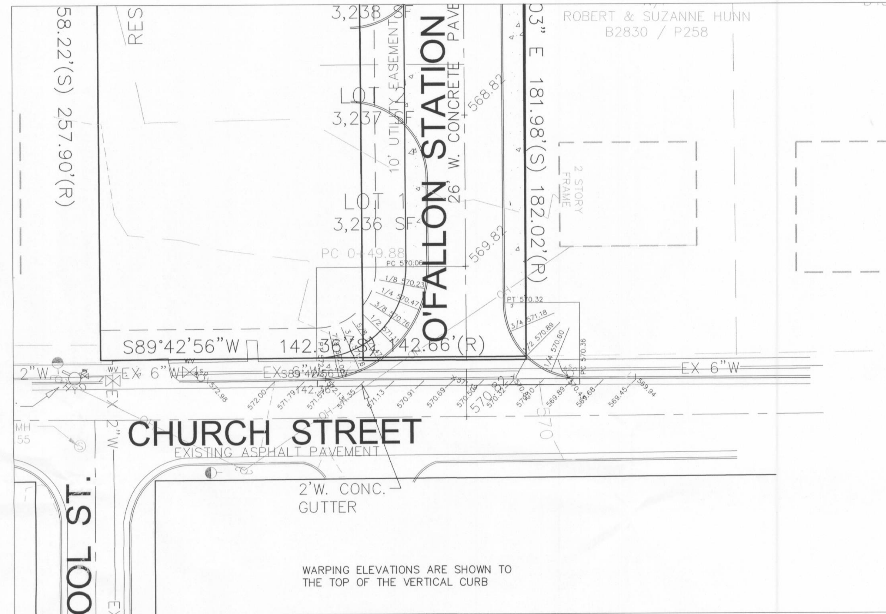
WARPING DETAIL FOR INTERSECTION OF CHURCH ST. AND O'FALLON STATION DR. SCALE: 1:20
