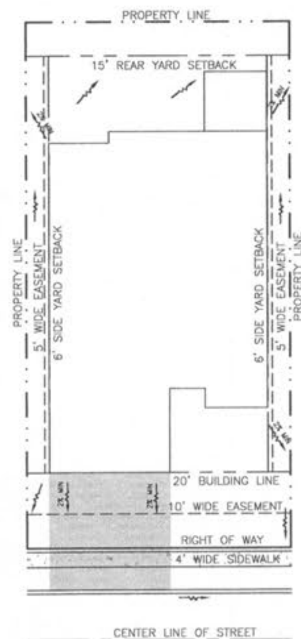
1 TYP. LOT FLOW PATTERN DETAIL SCALE: N.T.S. REF. DWG.
