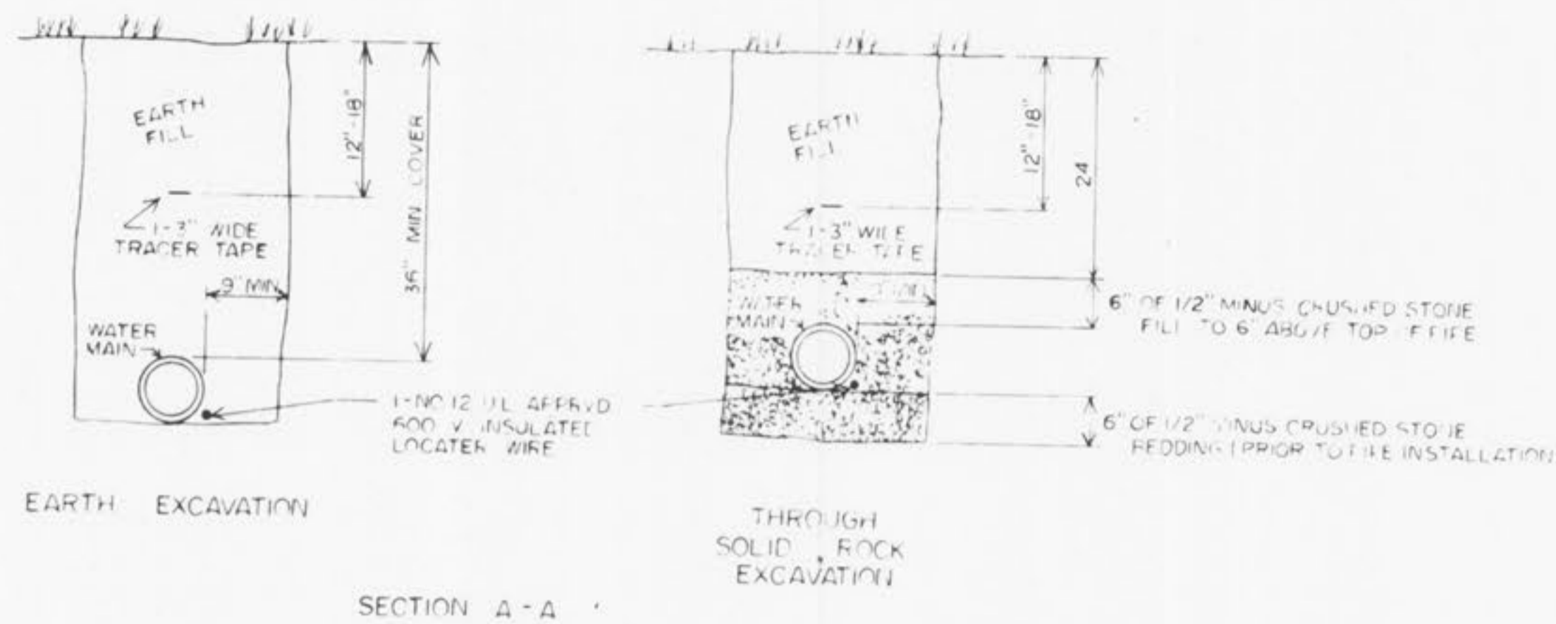
TYPICAL WATER MAIN INSTALLATION DETAILS NO SCALE
