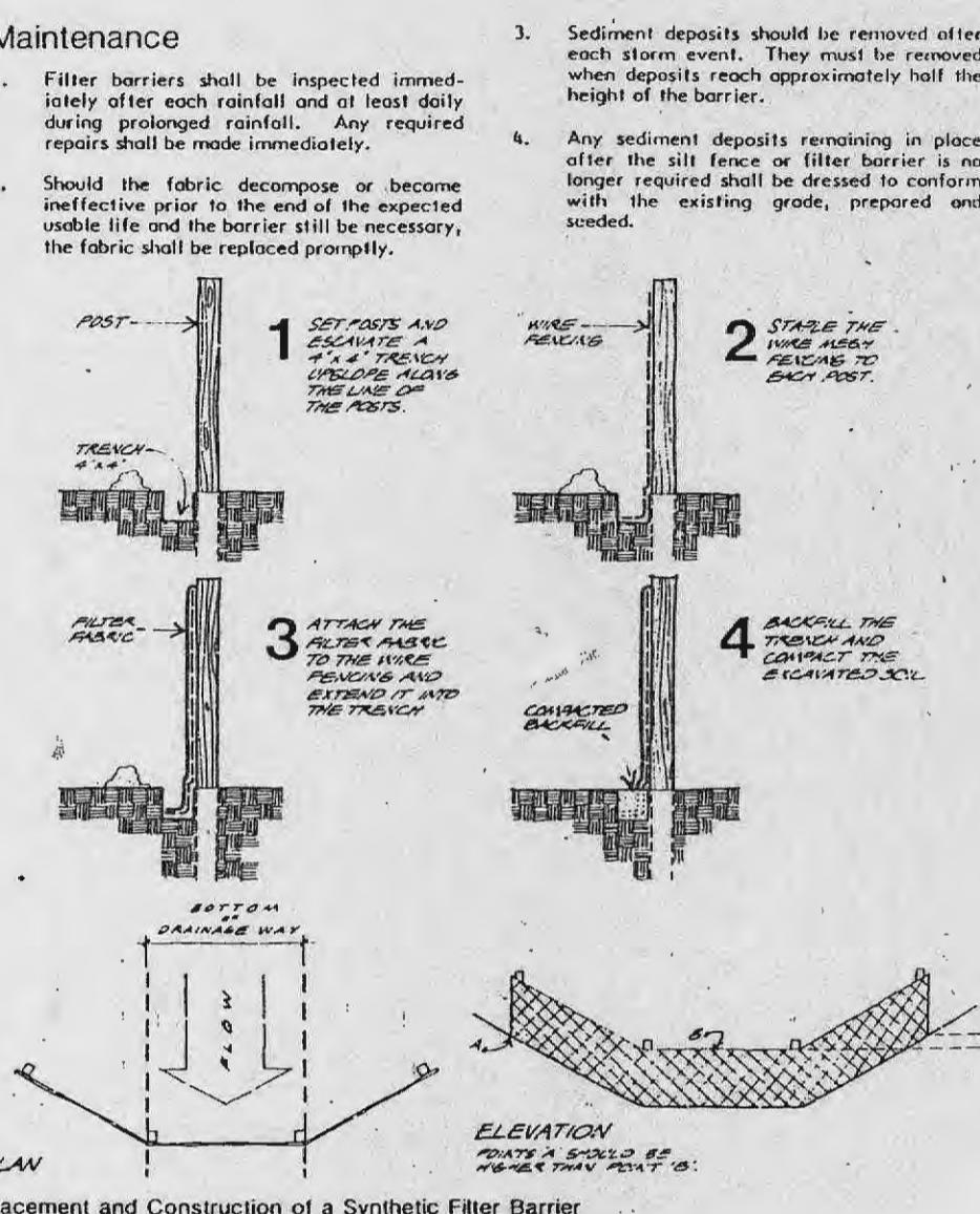
Placement and Construction of a Synthetic Filter Barrier
