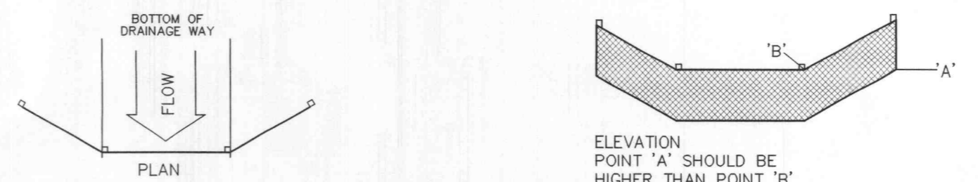
SILTATION FENCE DETAIL
