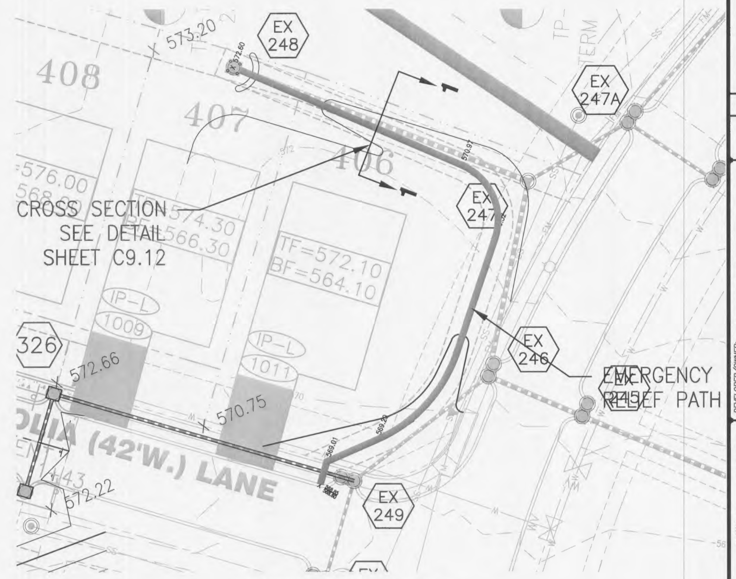
4 EMERGENCY SPILLWAY SCALE: 1"=20' REF. DWG.
