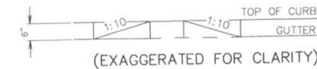
TYPICAL HC RAMP - ELEVATION
