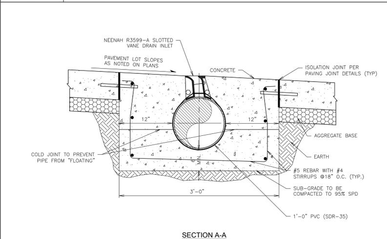
**F11** SLOTTED VANE DRAIN INSTALLATION CROSS SECTION "A-A" NTS SN: DD006A007
