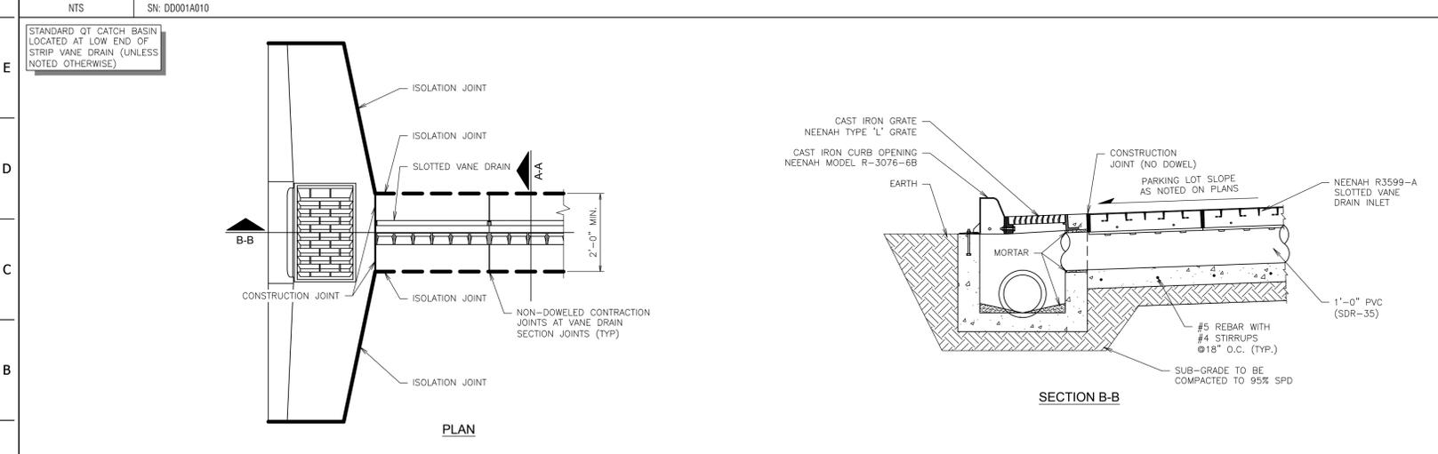
**A1** SLOTTED VANE DRAIN INSTALLATION @ CATCH BASIN DETAIL NTS SN: DD004A005
