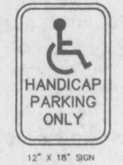
12" X 18" SIGN STANDARD SIGN FACE, STANDARD HIGHWAY DEPARTMENT, OR CITY STREET DEPARTMENT GAUGE. BLACK OR BLUE LETTERING. GALVANIZED STEEL POST 5'-6" LONG, SET 5'-0" INTO GRADE. SET BOTTOM OF SIGN 5'-0" ABOVE FINISHED GRADE. HANDICAP PARKING SIGN NO SCALE
