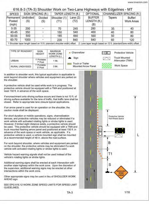
ON SIDE ROADS WITH POSTED SPEED OF 45 MPH OR GREATER, SIGNS SHALL BE PLACED 150 FT. IN ADVANCE OF INTERSECTION WITH MAINLINE.
