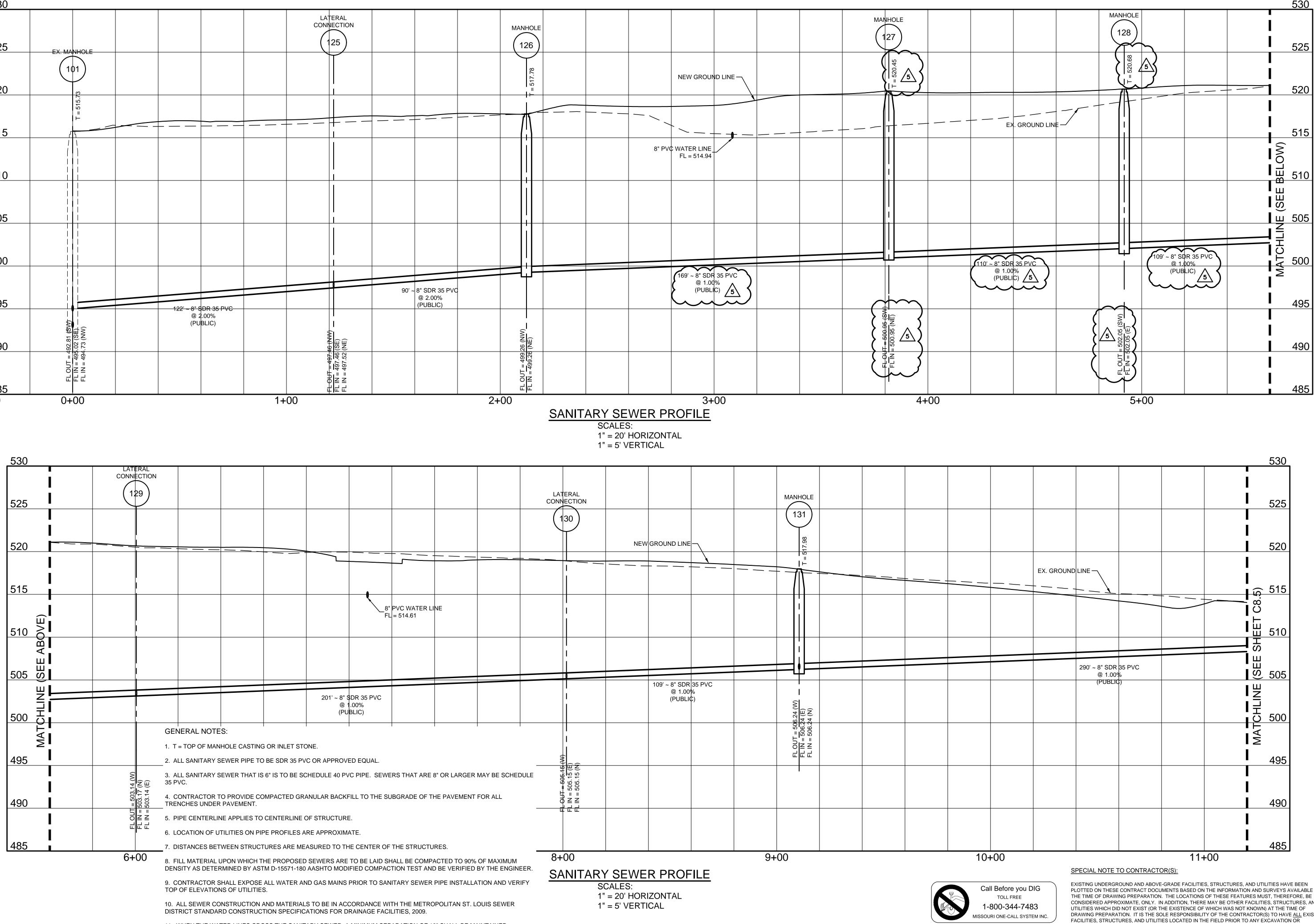
11. WHEN THE WATER LINES CROSS THE SANITARY SEWER, A MINIMUM SEPARATION OF 18" SHALL BE MAINTAINED BETWEEN WATER LINE AND SANITARY SEWER.
