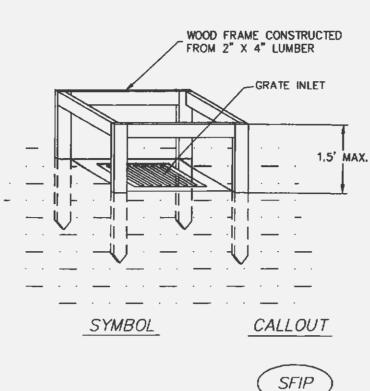
SILT FENCE INLET PROTECTION
