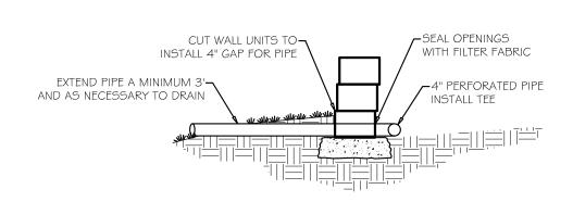
PERFORATED PIPE OUTLET - TYPE I NOT TO SCALE
