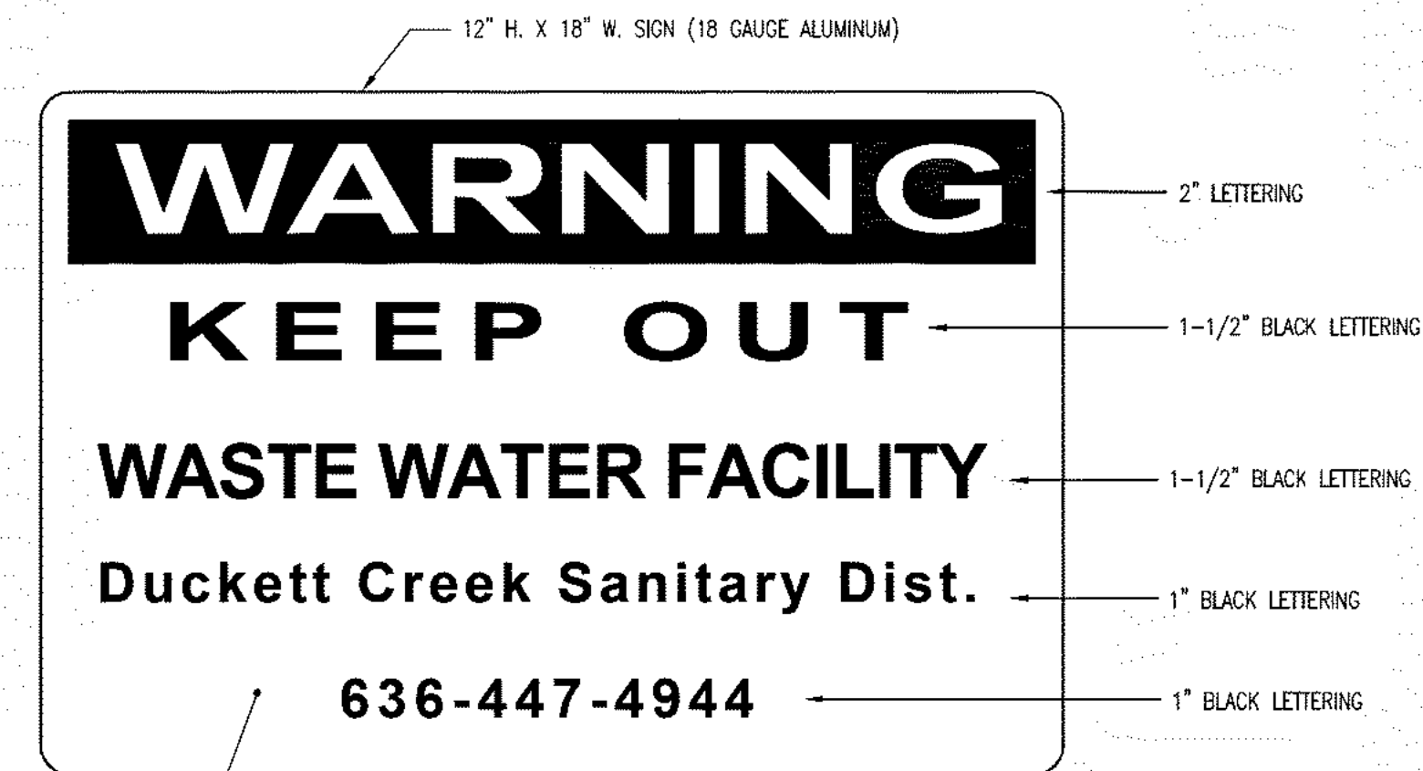
4 REQUIRED WARNING SIGN DETAIL NTS
