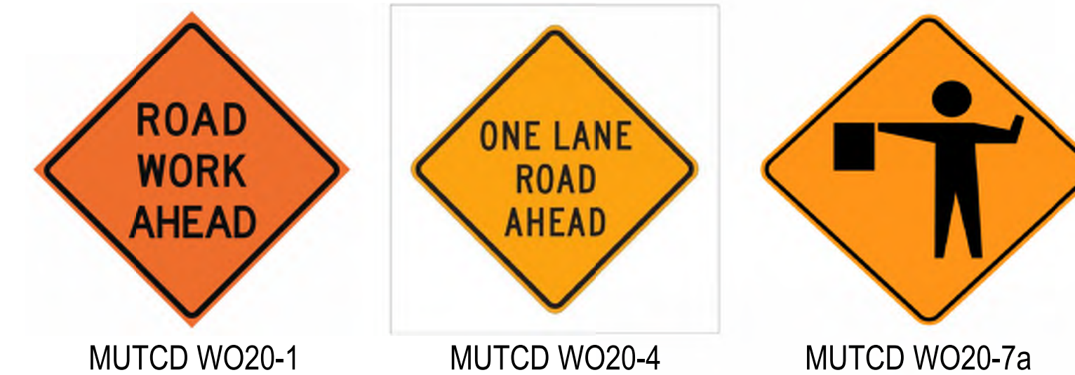
SINGLE LANE CONSTRUCTION TRAFFIC SIGNAGE
