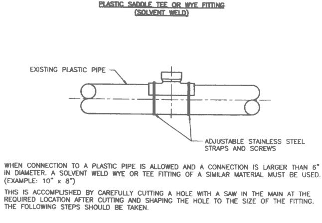
1. CLEAN AND DRY BOTH INSIDE THE SADDLE WYE SURFACE AND PIPE SURFACE TO BE SOLVENT CEMENTED. 2. IMPORTANT: APPLY A LIBERAL, HEAVY COAT OF ONE-STEP SOLVENT CEMENT TO THE INSIDE SURFACE OF THE SADDLE WYE AND TO THE EXTERIOR WELDING SURFACE TO THE PIPE.
