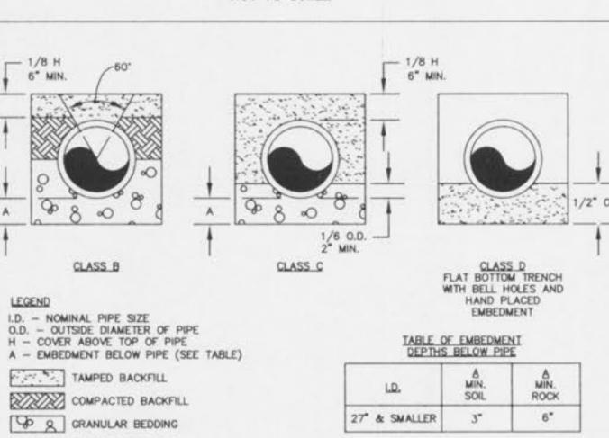
GRANULAR BEDDING SHALL BE CRUSHED ROCK OR PEA GRAVEL WITH NOT LESS THAN 95% PASSING 1/2" (95% PASSING 3/4" FOR 30" AND LARGER PIPE) AND NOT LESS THAN 95% RETAINED ON A #4: TO BE PLACED IN NOT MORE THAN 6" LAYERS AND COMPACTED BY SLICING WITH A SHOVEL OR VIBRATING.
