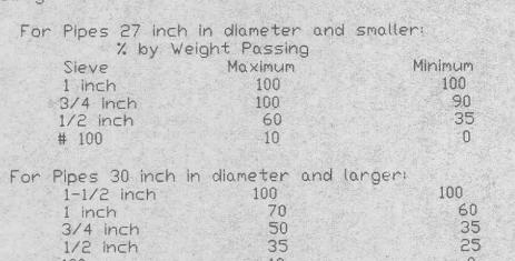
Backfill Aggregate: Backfill Aggregate shall be crushed limestone and screenings and be 3/4 inch minus.
