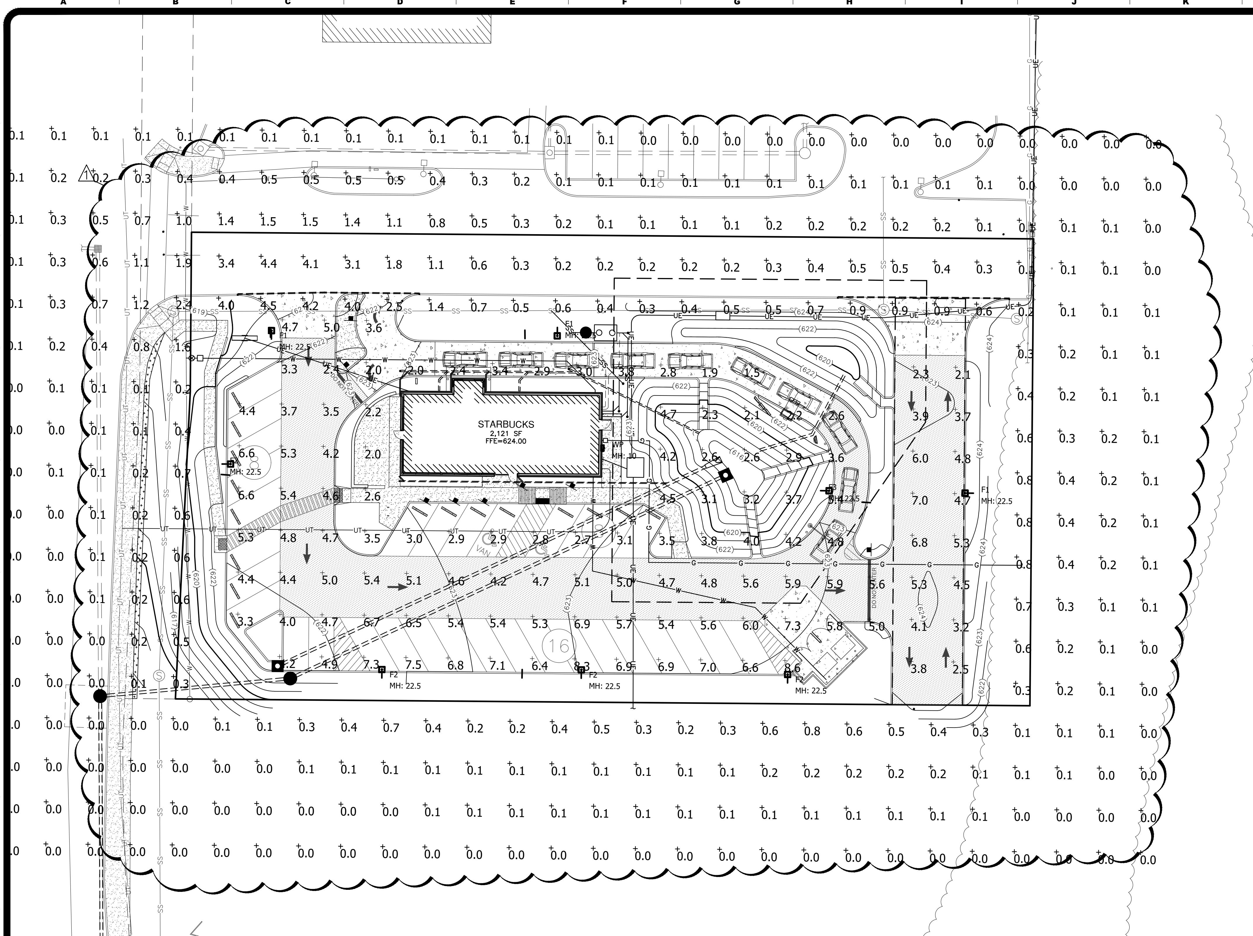
POLE FIXTURES MOUNTED ON 20' POLE & 2.5' BASE
