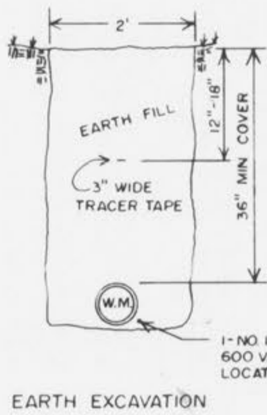
TYPICAL WATER MAIN TRENCHING DETAIL NO SCALE
