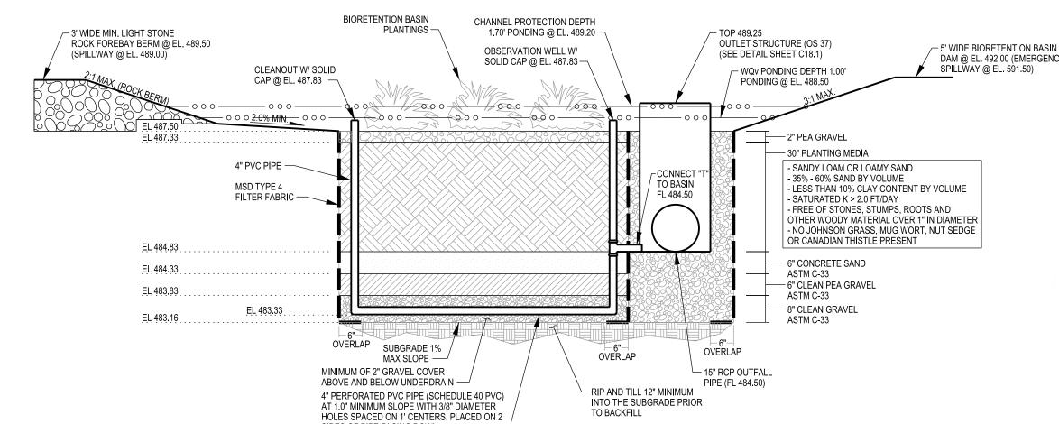
BIORETENTION (F-6) TYPICAL SECTION:
