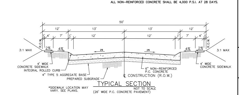
ALL NON-REINFORCED CONCRETE SHALL BE 4,000 P.S.I. AT 28 DAYS.
