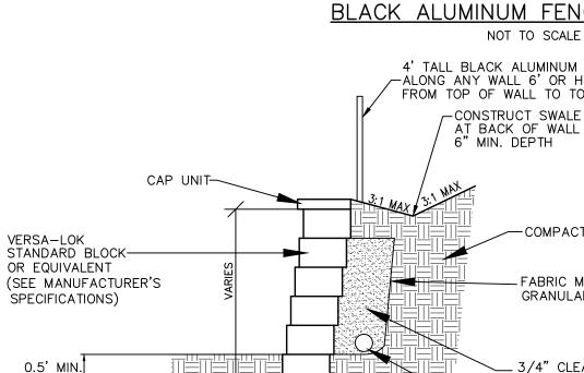
The use of High Density Polyethylene Corrugated pipe A.D.S. N12 or Equal will be permitted
