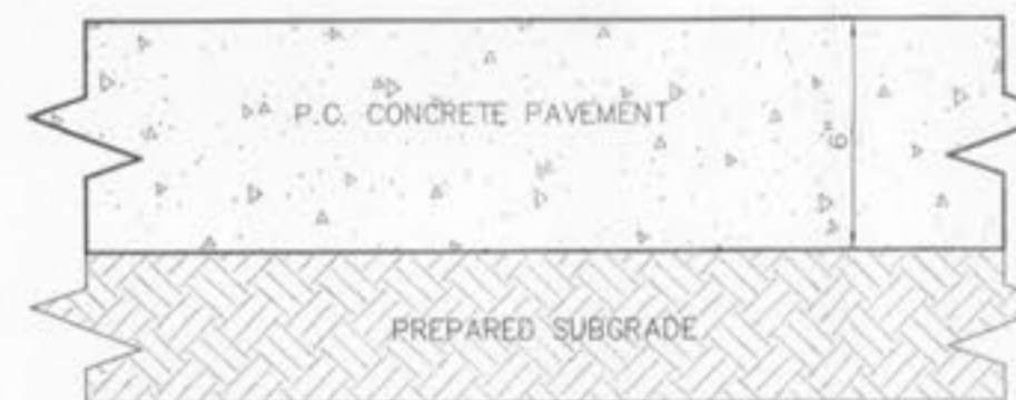
TRASH ENCLOSURE PAVEMENT DETAIL NOT TO SCALE
