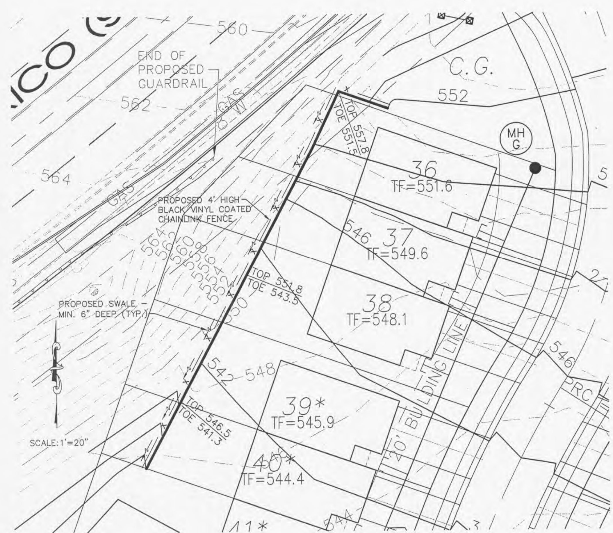
MODULAR BLOCK RETAINING WALL #1 PLAN VIEW
