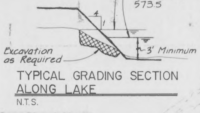
TYPICAL GRADING SECTION ALONG LAKE N.T.S.
