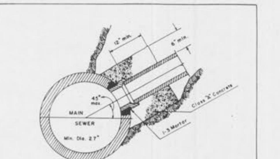
Note: The opening shall be cut by the contractor in a sufficient size to permit inserting a tee saddle or short length of pipe of the required elevation and angle to allow at least two (2) inches space around the pipe. This space will be solidly filled with 1-3 cement-sand mortar and the new pipe neatly trimmed and pointed up with mortar to the level of the main sewer.
