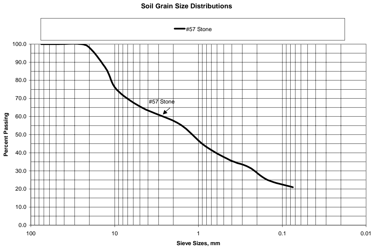
Figure B-1. Infill grain size distribution curve
