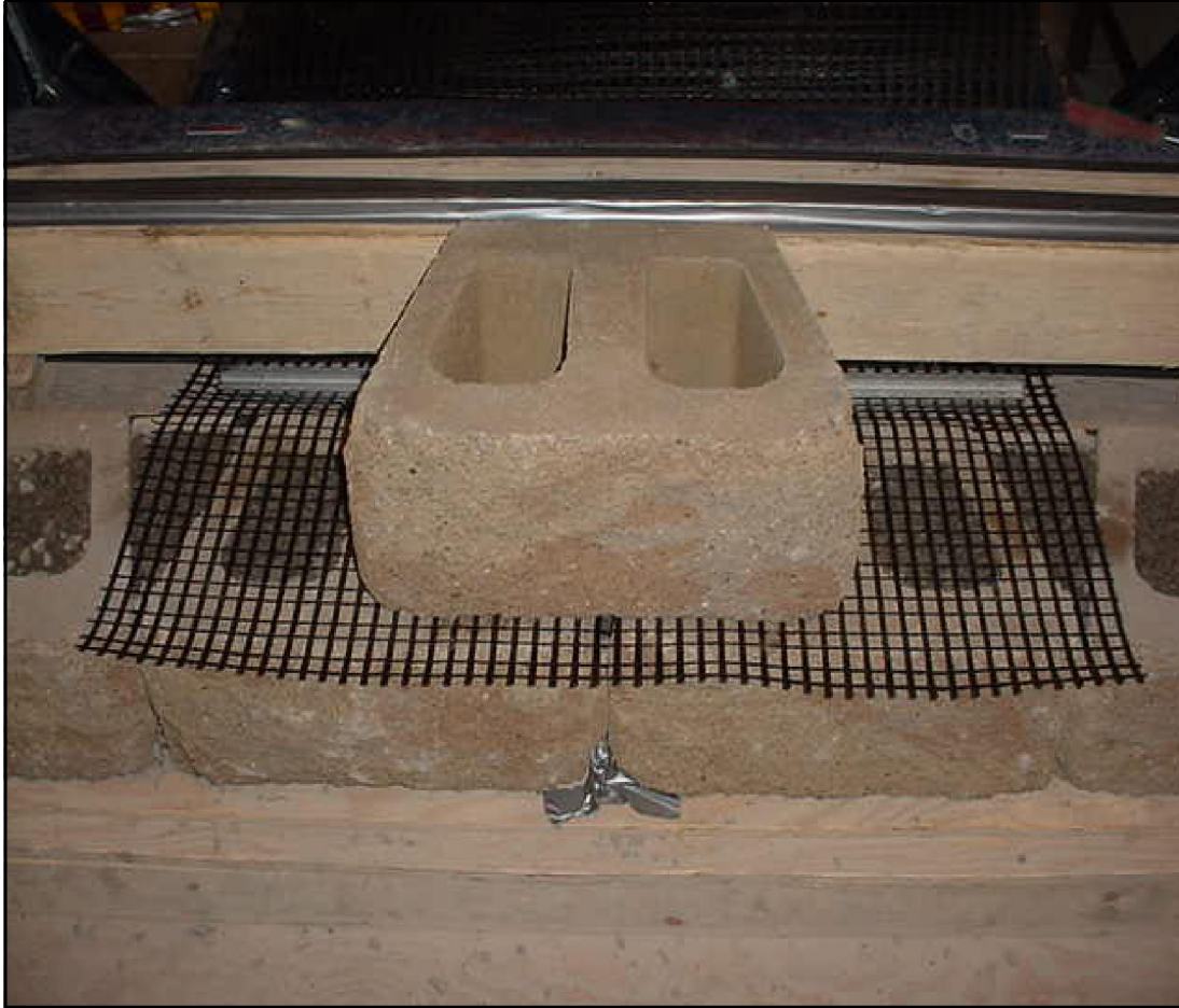
Figure 2: Photograph of Diamond Pro block units in the connection test apparatus
