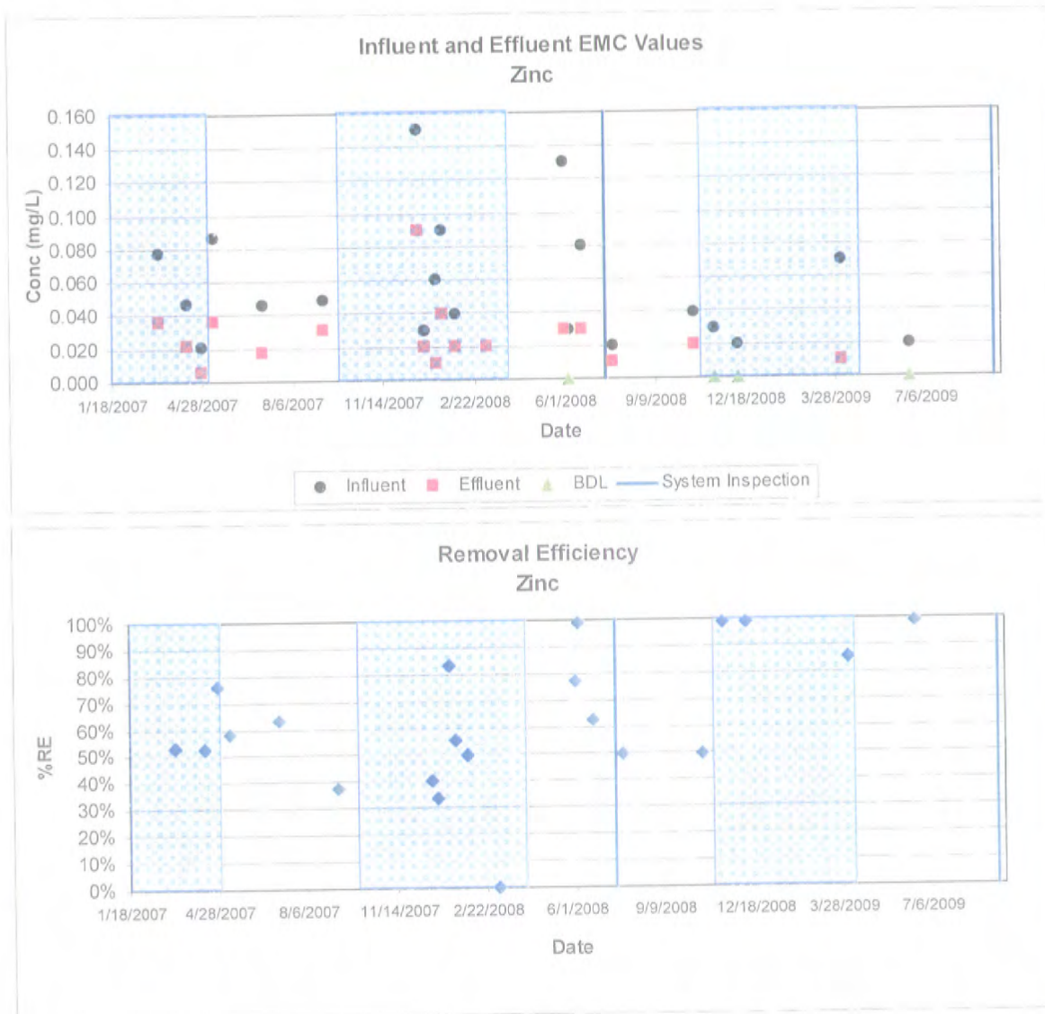
Figure 8: Total Zinc Event Mean Concentrations at influent and effluent locations and Removal Efficiencies for 21 storm events of the Isolator Row®. A 6-month winter period (Nov-April) is displayed in blue.
