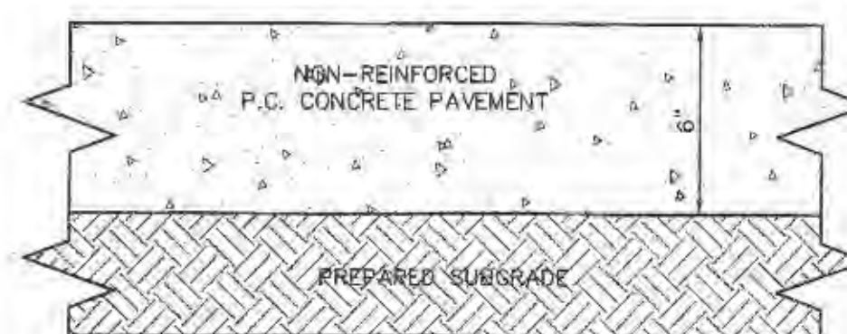
DRIVEWAY PAVEMENT DETAIL NOT TO SCALE
