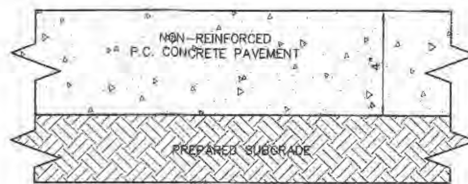
SIDEWALK DETAIL NOT TO SCALE
