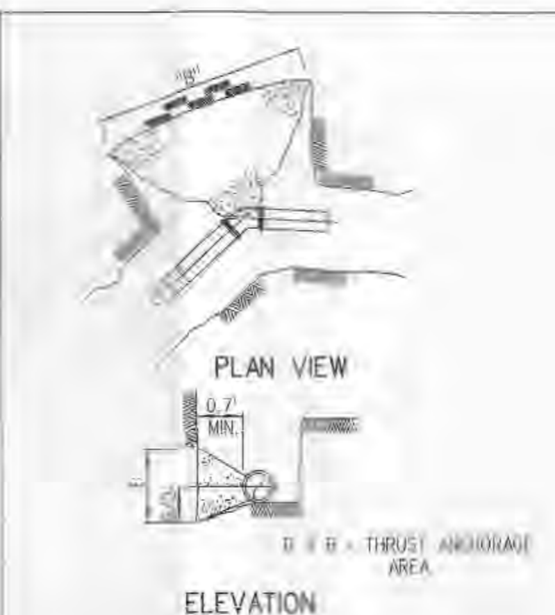
THRUST BLOCK FOR HORIZONTAL OFFSETS
