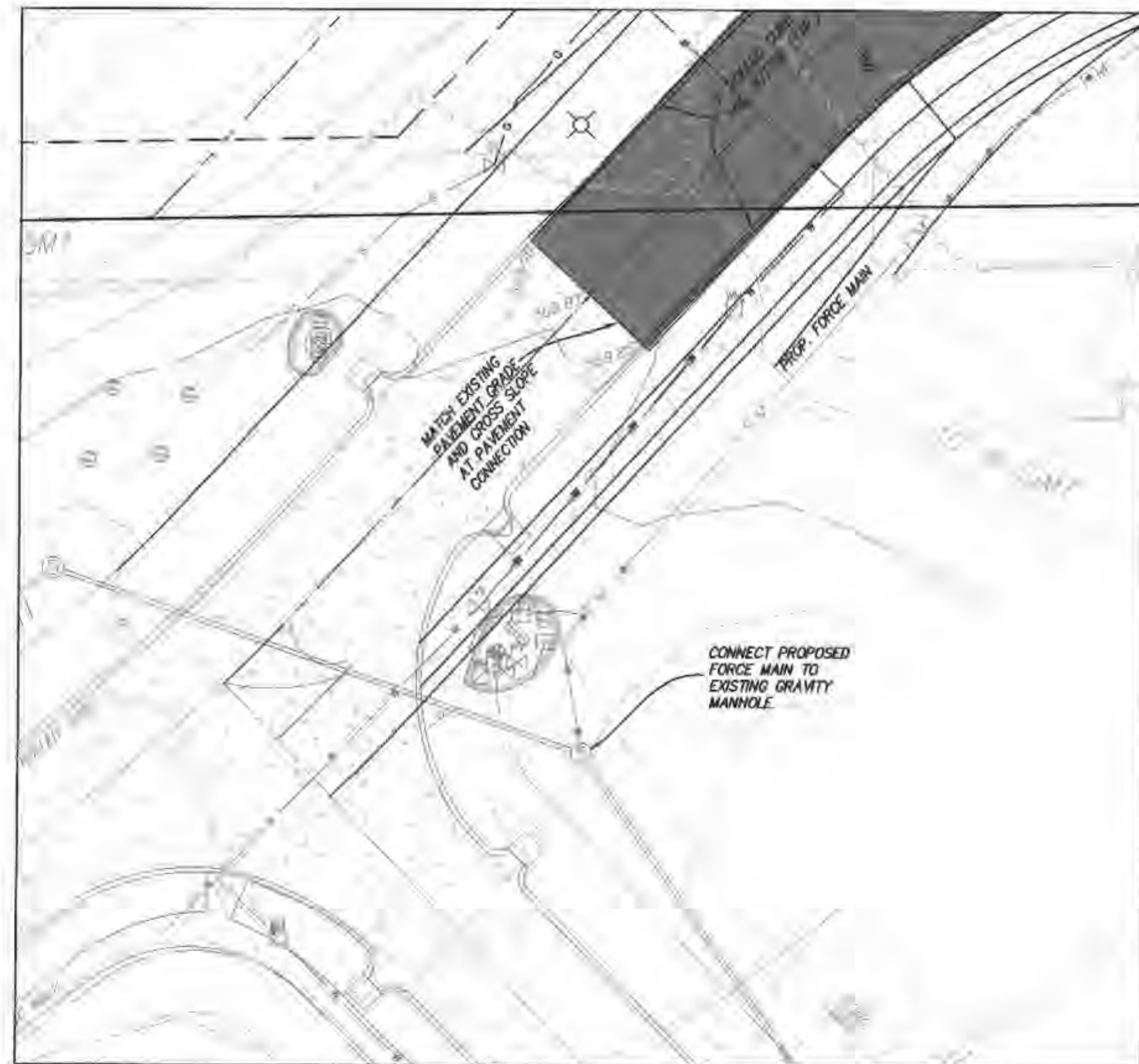
FORCE MAIN CONNECTION TO EXISTING MANHOLE SCALE: 1"=20'
