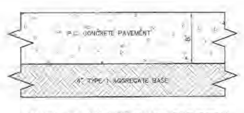
TRASH ENCLOSURE PAVEMENT DETAIL NOT TO SCALE
