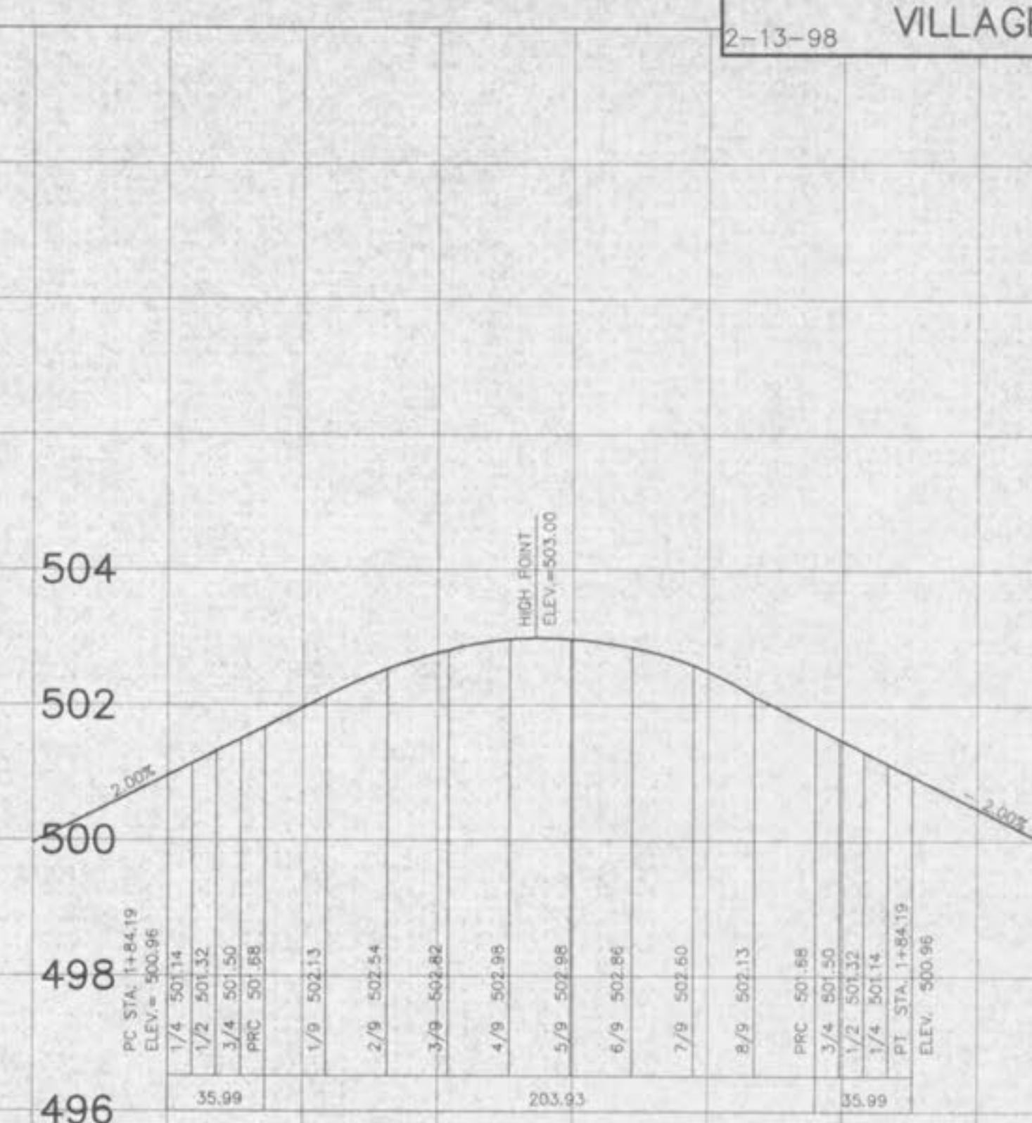
FALLON PASS CUL-DE-SAC WARPING TOP OF CURB ELEVATION
