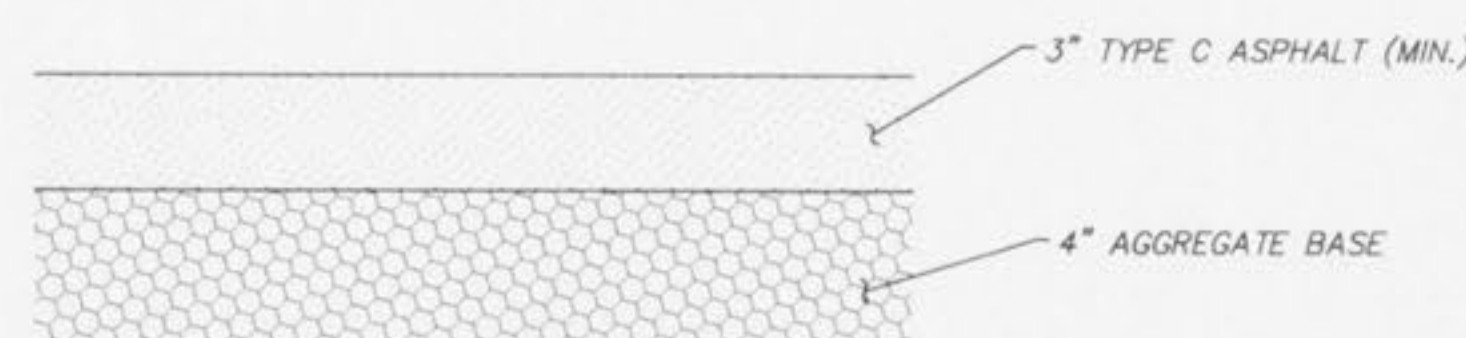
MULTI-USE TRAIL DETAIL (MINIMUM 4' WIDE) NOT TO SCALE
